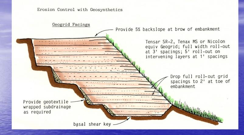
Section through a MSE embankment with a 1:1 (45 degree) finish face inclination. The embankment utilized false layers every 12 inches, extending just 5 feet into the slope (from Rogers, 1992)
