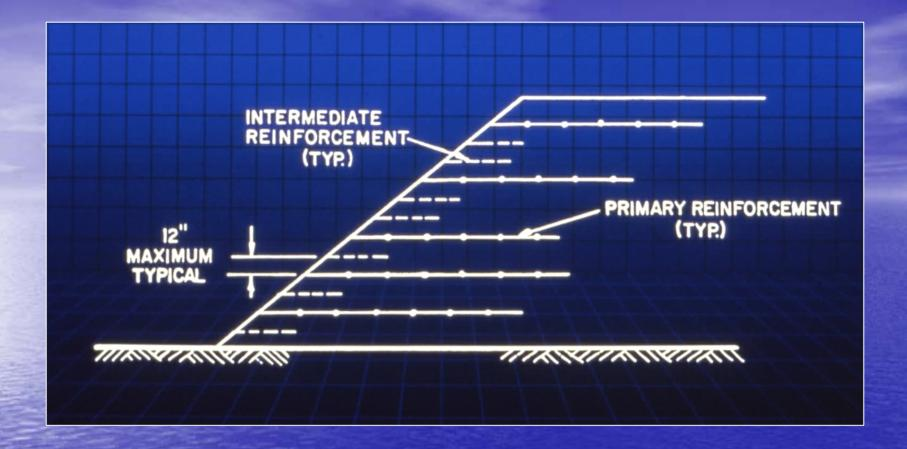
We can make embankments slopes as steep as we desire by using "false layers," of geotextiles, between primary reinforcement layers of mechanically stabilized embankments (MSE).
