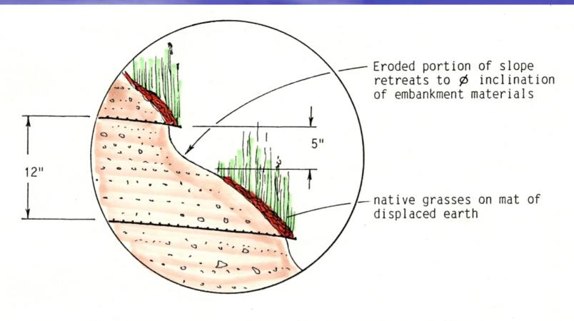
Detail view of the erosion which can be expected to occur between Geogrid layers. The effective slope height is reduced to 12" by embedment of the Geogrid.
