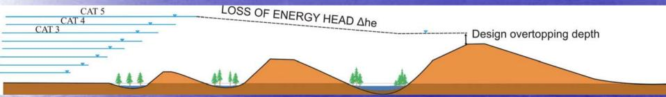
Green segmented levee protection systems could be tweaked for any number of variables; including a *design overtopping depth* to accommodate low frequency events; without using as much earth fill as conventional embankments.
